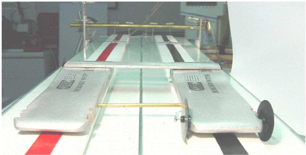
**Figure 3** - Front view of car configuration E3. Only the 2 outside rear wheels and the rightmost front wheel are touching. The inside front wheel is only for center strip guiding if needed. The rod in the rear is replaced by an aluminum bar that keeps the body insides from drooping at an angle.
