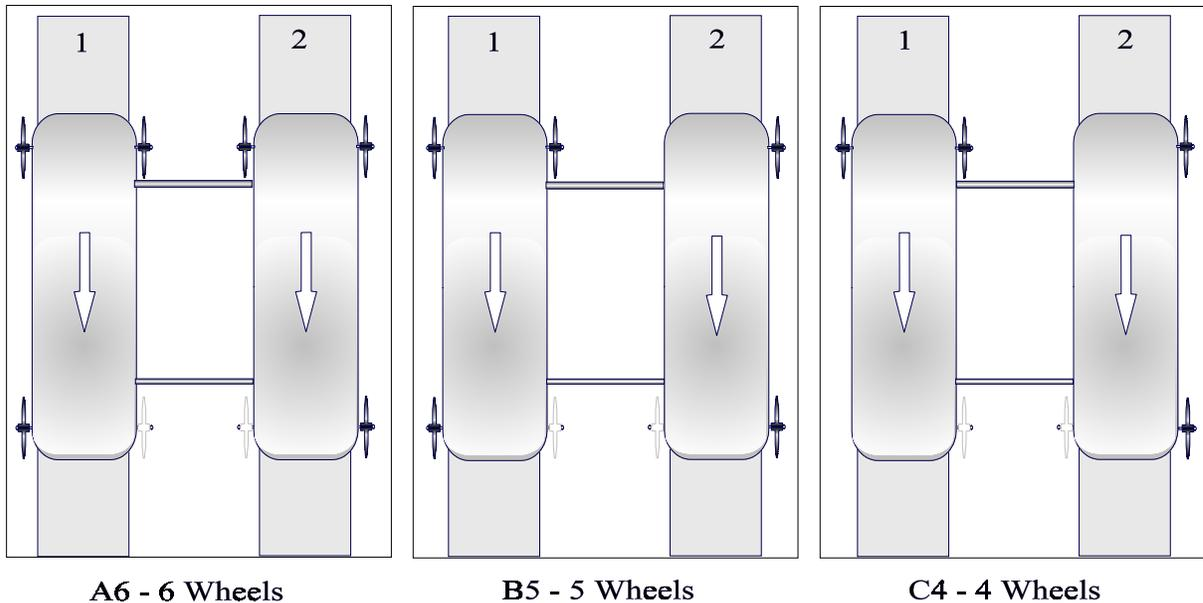
**Figure 2** - Top view of the dual car with A6 - 6 wheels supporting car, B5 - 5 wheels supporting car, and C4 - 4 wheels supporting car. The Shaded light wheels do not touch track surface.
