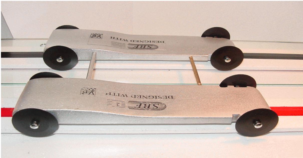
**Figure 1** - Side view of the dual car that weighs 10 oz. The 2 inside front wheels do not touch. The front brass rod is 3/32" ID covering 3/32" wood dowels protruding from each car body. The rear aluminum rod is 1/8" ID to allow enough play for each of the 4 rear wheels to be firmly planted.
