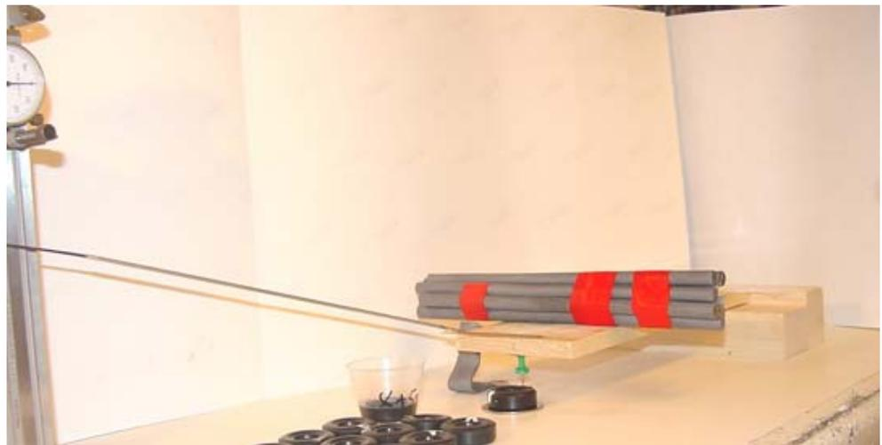
**Figure 1** - The apparatus for testing the hardness of polystyrene pinewood derby wheels.
